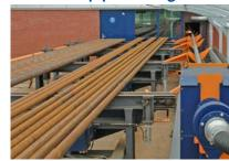
The large pipe buffer allows the loading of multiple pipes (bundle) at once. The infeed of pipes into the cutting cell occurs fully automatically.
