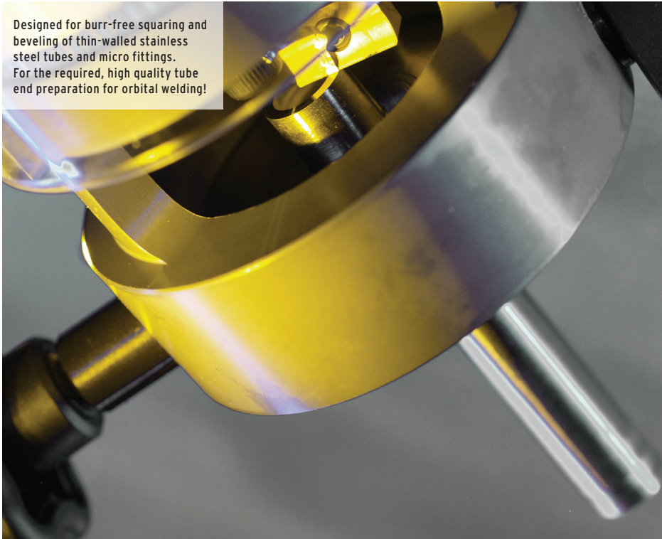
Precise clamping of tubes and micro fittings
