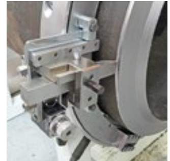
Newly designed slides with Rapid Retract feature
